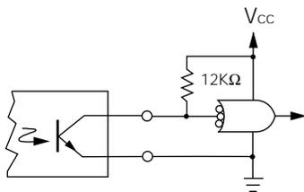
Note: Use smaller pull up resistor for higher speed.
