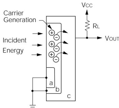
Thus a current flows from collector to base, causing a voltage drop across the load resistance ( $R_L$ ).
