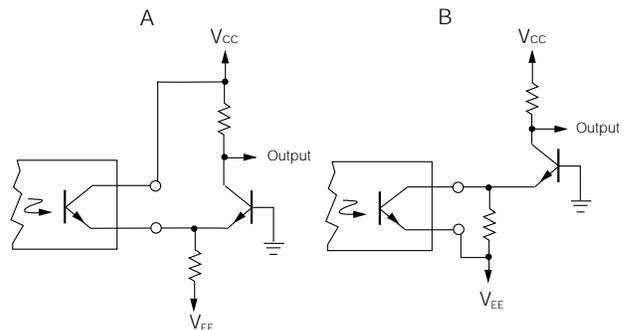
The circuit will work equally well either way, with a phase inversion between the two. Obviously a PNP transistor would work as well.
