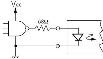
Note: Can omit resistor for about 15 mA into diode.
