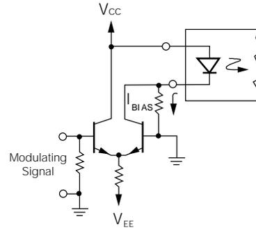
Sensing in linear applications can be done in several ways depending on the requirements. For high frequency performance, the phototransistor should be operated into a low impedance input current amplifier. The simplest such scheme is a grounded base amplifier.
