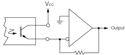
Note that in all cases the output can be taken from either the collector or the emitter of the phototransistor depending on the polarity desired. The operating speed is the same in either case.
